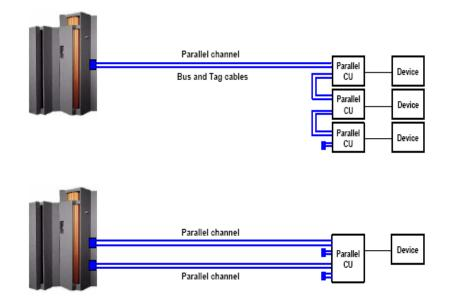
The maximum data rate of the parallel channel was 4.5 MB, the maximum distance was 122 meters (400 ft).
