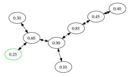
Figure: Put example from node with ID 0.25 inserting data identified by the ID 0.93
