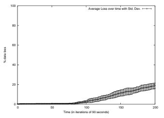
Figure: Graph showing average data loss over 5 runs with 800 nodes and 2 attack nodes using 8 bad locations with the attack starting after about 2h.
