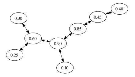
Figure: A GET request from node 0.90 searching for data with identifier 0.22 (which is stored at node identified by 0.25)
