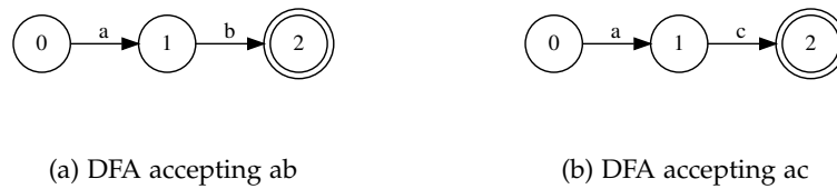
Figure 3.2: DFAs for the regular expressions ab (a) and ac (b) that should be merged in the DHT.
