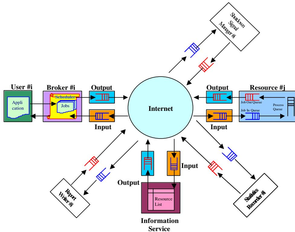
Figure 3. A flow diagram in GridSim based simulations.
