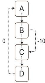
**Figure 10:** Example of unsatisfiable message constraints. Each node is annotated with its input and output rate. Messages are shown by dotted arrows, drawn from sender to receiver with a given latency. The constraints are satisfiable in isolation, but unsatisfiable in combination.
