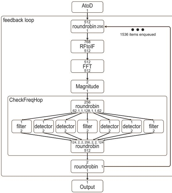
**Figure 13: Stream graph of frequency hopping radio with control messages implemented manually.** A feedback loop connects the detectors with the RFtoIF stage, and an item is sent on every invocation to indicate whether or not a message is present. The latency and periodicity of message delivery are governed by the data rates and the number of items on the feedback path.
