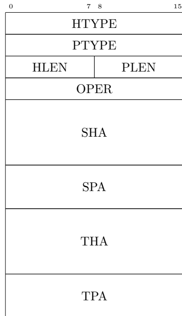
Figure 5: ARP; HTYPE for Ethernet is 1, PTYPE for IPv4 is 2048, EtherType: 0x0806.
