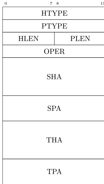
Figure 3: ARP; HTYPE for Ethernet is 1, PTYPE for IPv4 is 2048, EtherType: 0x0806.
