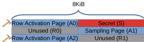
(b) Single-sided Rambleed. Here, the sampling page (A1) is neighbored by the secret-containing page (S) on a single side.
