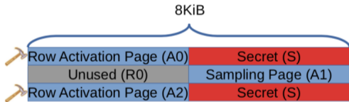
(a) Double-sided Rambleed. Here, the sampling page (A1) is sandwiched between two copies of S.
